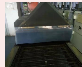
Replacing the draft shield of the tunnel furnace
